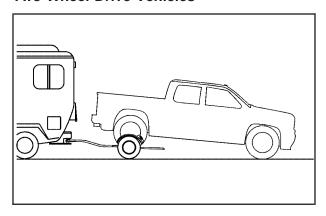
Use the following procedure to dolly tow a two-wheel-drive vehicle from the rear:
